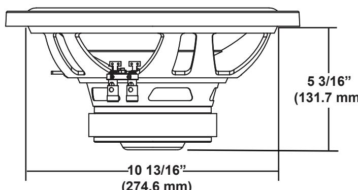
**Recommended Power Rating of 125 - 250 Watts RMS**
